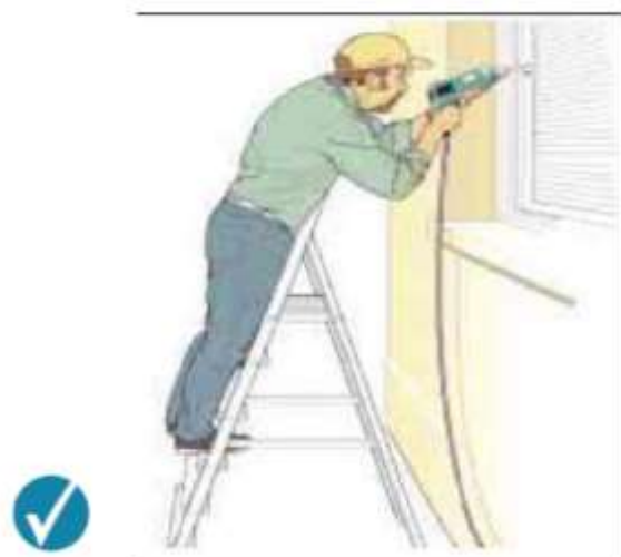
Correct – steps facing work activity
